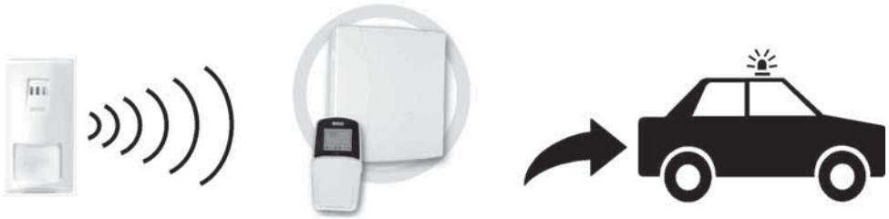
A sensor detects. ►► The control system is alerted. ►► An alarm is generated and the monitoring service is notified.
