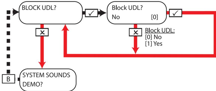
This function will block any attempt made to dial into the control panel to upload and download information if enabled.
