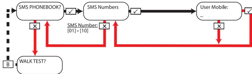
**NOTE:** Mobile numbers can be entered with or without an international dialling code (e.g. +44). If you need to enter an international dialling code to send the key to a foreign SIM card – use the **A** key to enter the '+' symbol.
