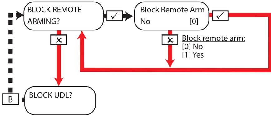
This function will block any attempt made to arm or disarm via the UDL software if enabled.
