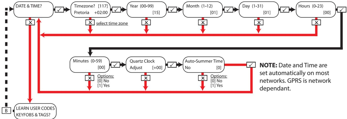
**NOTE 1 - Quartz Clock Adjust:** If the clock is losing time, this function is used to compensate for the minutes being lost and therefore making the control panel show the true time. The adjustments are programmed in minutes, so for example if the time gains 2 minutes, select -02 on this option. If the time loses 4 minutes, select +04 on this option etc.
