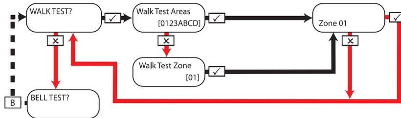
**NOTE:** When walk testing areas - walk around to trigger all of the zones in the selected areas until the panel displays 'Walk Test Zones Completed'. When using the 'walk test zone' option to choose a specific zone to test - the keypad will make an audible 'beep' each time the zone is triggered.
