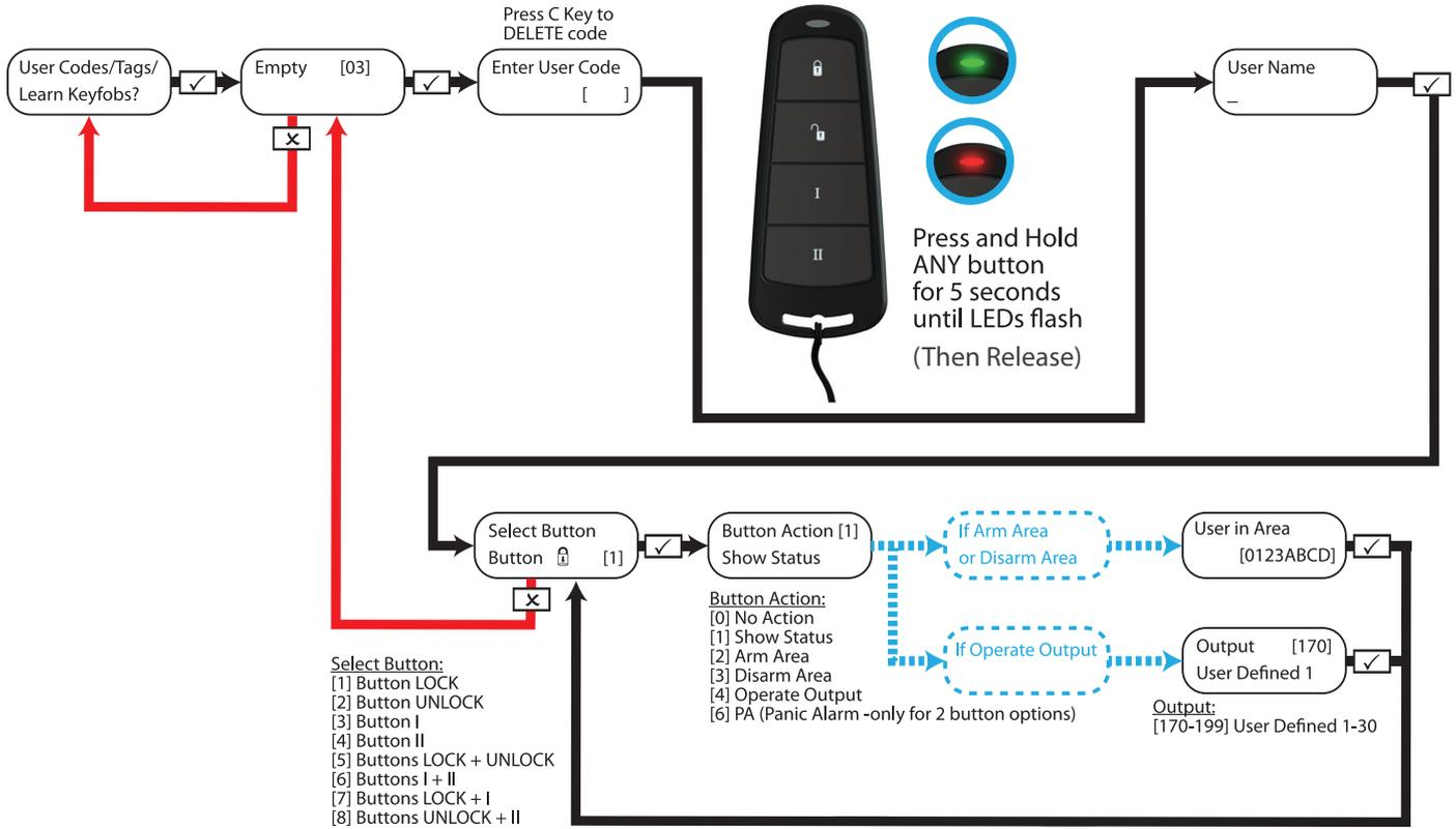
**NOTE:** Keyfobs can only be learnt to the **PCX46 App** control panel if a PCX-RIX32-WE is installed (Enforcer wireless expander)
