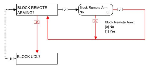
This function will block any attempt made to arm and disarm the UDL software if enabled.
