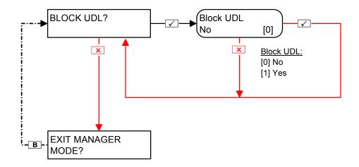
This function will block any attempt made to dial into the control panel to upload and download information if enabled.
